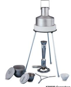
K80030 Conradson Carbon Residue Apparatus
