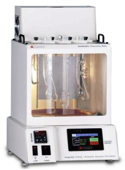
K23802 Digital High Temperature Kinematic Viscosity Bath (HKV4000)
